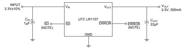
Note:  $\overline{SD}$  and  $\overline{ERROR}$  pins must be pulled high through a 10k $\Omega$  pull-up resistor. Connect the  $\overline{ERROR}$  pin to ground if this function is not used.
